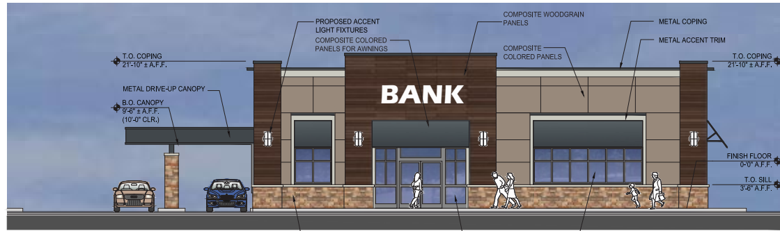
PROPOSED BUILDING FACADE - WEST (SCHEME 2)
