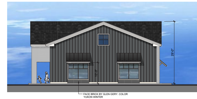
PROPOSED SIDE (NORTH) ELEVATION- SCHEME 1 SCALE: 1/16" = 1'-0"
